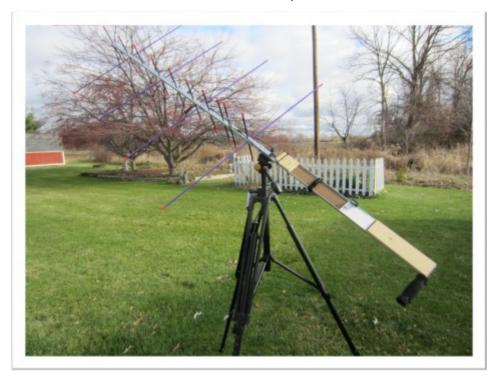
They both have a break down option to transport/backpack. The tripod is necessary for the Alaskan due to weight, and is preferable to controlling the antenna with one hand on a 15 minute pass while adjusting the radio in the other and writing down call signs with the third.
